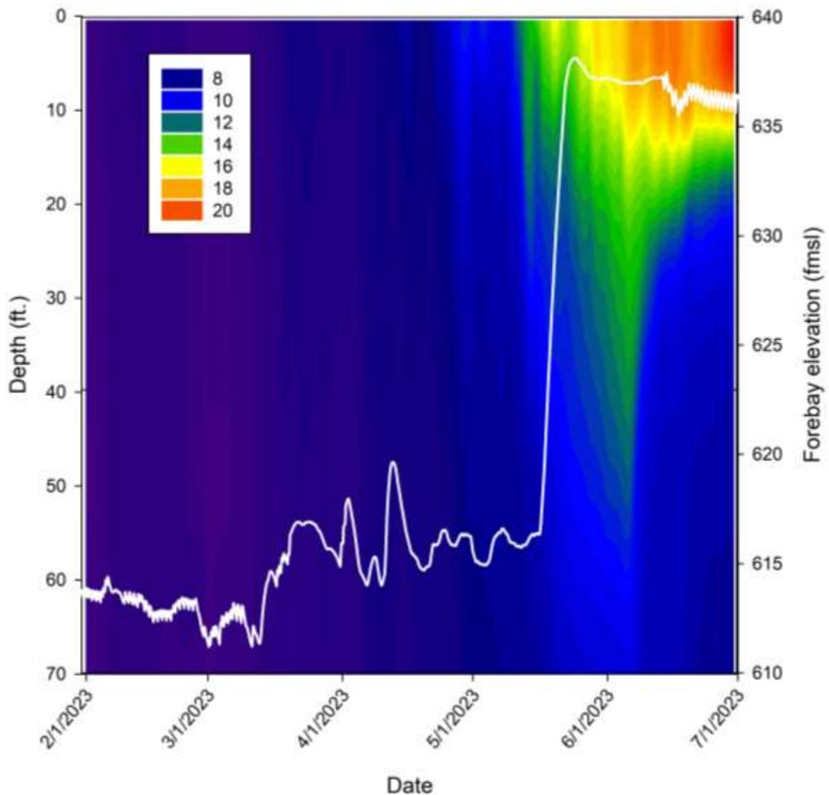
Figure 3-10. Daily average forebay elevation (solid white line; right axis) and temperature ( $^{\circ}\text{C}$ ) at depth (contour plot; left axis) in the Foster Forebay from February 1 through June 30, 2023.
