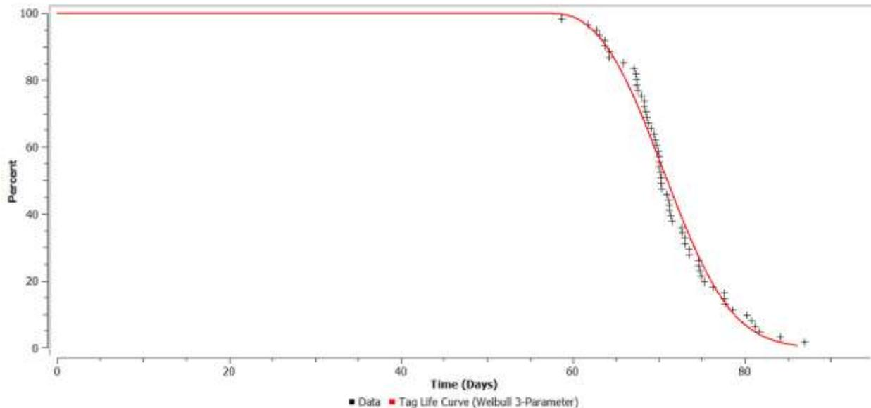
Figure 3-1. Weibull three parameter model fit to the observed tag life of radio tags used during the spring survival study conducted at Foster, 2023.
