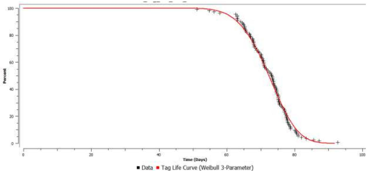
Figure 3-3. Weibull three parameter model fit to the observed tag life of radio tags used during the fall survival study conducted at Green Peter and Foster, 2023.
